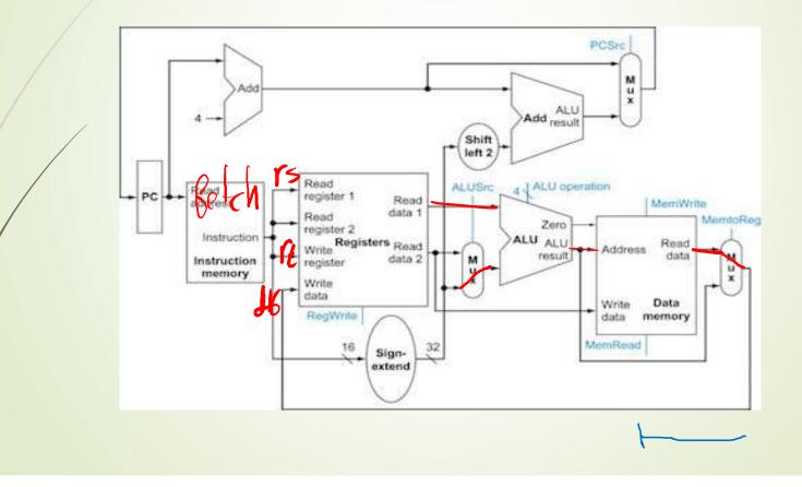
The single-cycle datapath conceptually described in this section *must* have separate instruction and data memories, because \_\_\_\_\_.
